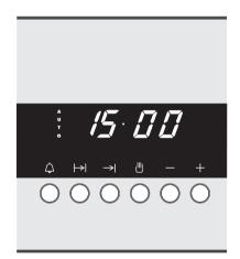
**i** If the appliance has been isolated from the mains, e.g. due to a power failure, the time display will flash again. In this case reset the time again, as described above.
